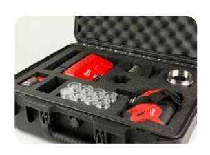
Field Sample Pulverizer and Press Kit in Case
