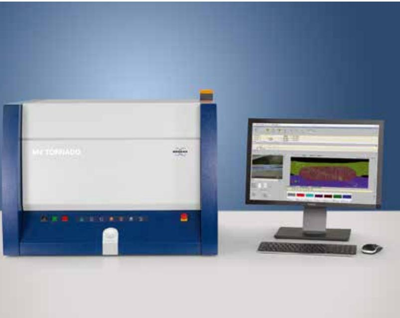
Micro-XRF is the method of choice for highly sensitive and non-destructive elemental analysis of diverse samples, including inhomogeneous and irregularly shaped specimens.
